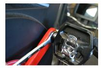
2. Using an 8mm Allen wrench, remove the bolt from the crank arm.
