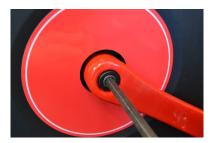
3. Using a 22mm crank puller, remove the crank arm from the frame.
